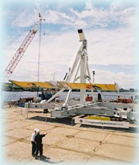
Oscillating Hydrofoil (Stingray) Source: The Engineering Business
